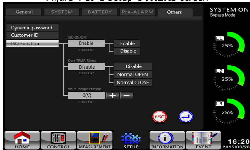
Figure 4-19-2 ISO function sub menu screen
