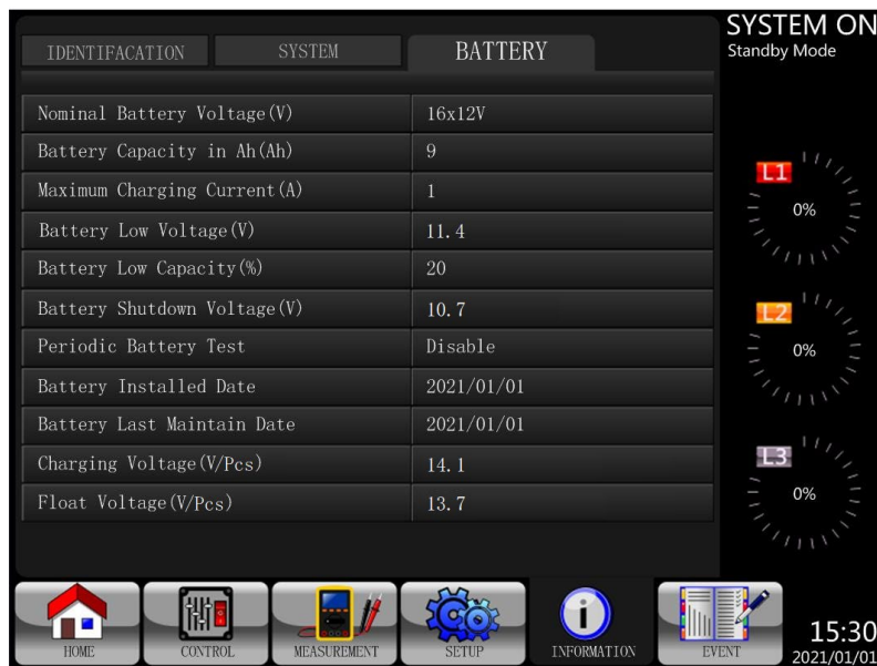
Figure 4-24 INFORMATION Battery screen page
