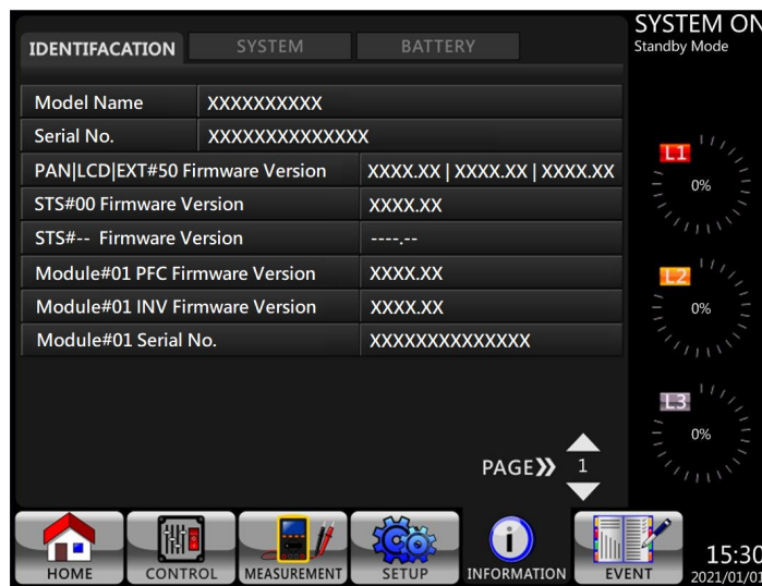
Figure 4-21 Identification screen page
