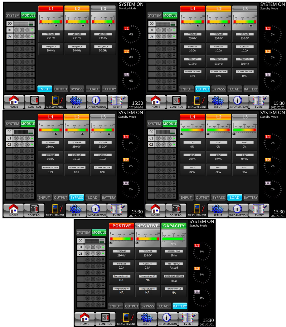
Figure 4-10 Module Measurement Screens
